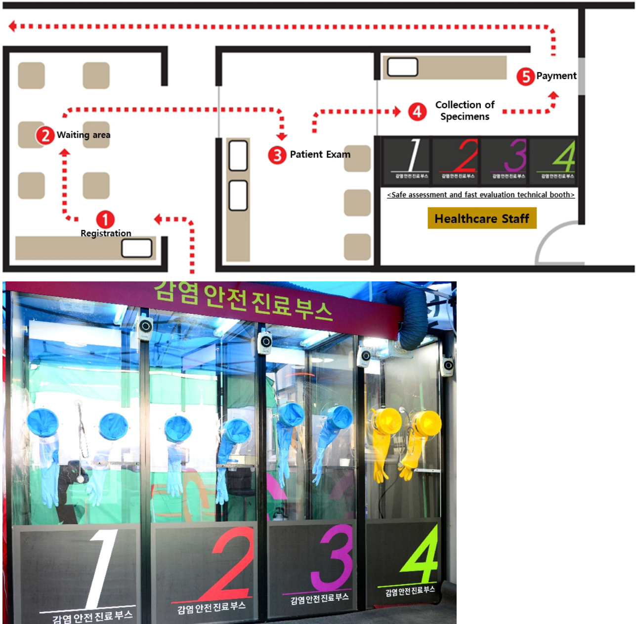
Fig. 2. The Walk-through (WT) test using the negative pressure booth. (Top) Flow diagram of the testing, and (Bottom) a picture of four "safe assessment and fast evaluation technical booths."
